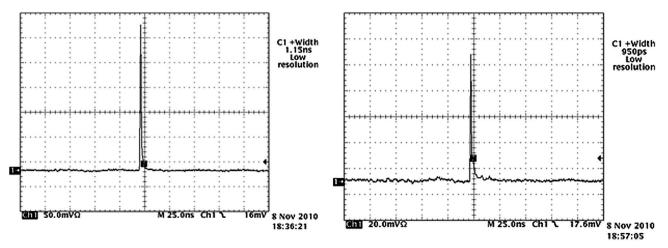
Fig. 5. Typical oscilloscope trace of the mid-infrared pulses at two different wavelengths. Left: 1.9 µm. Right: 2.2 µm.
