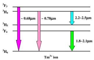
Fig. 7. (Color online) Energy diagram of  $Tm^{3+}$  ion. Some energy transitions that could be involved in the broadband supercontinuum generation process in this approach are indicated in the diagram.
