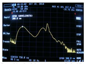
Fig. 8. (Color online) Red emission spectra in a Tm-doped fiber amplifier associated with the mid-infrared supercontinuum generation when pumped with a laser pulse at  $1.55 \ \mu m$ .
