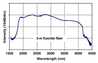
Fig. 10. (Color online) Spectral broadening in 3 m fluoride glass fiber.
