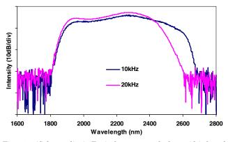
Fig. 4. (Color online) Typical spectra of the mid-infrared supercontinuum pulses measured by a monochromator at pulse repetition rate of 10 kHz and 20 kHz.
