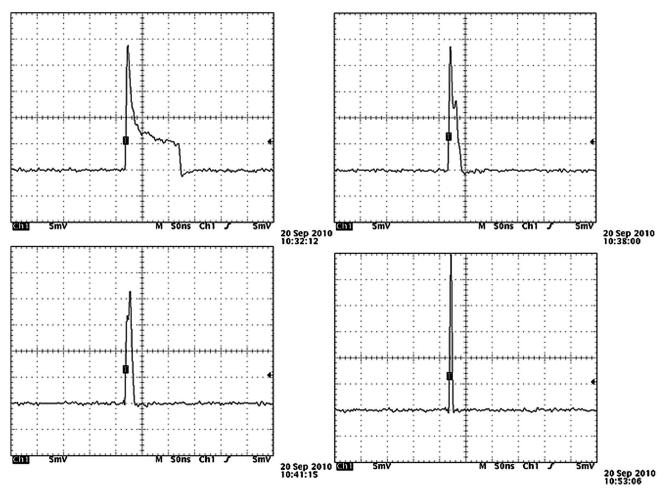
Fig. 3. Pulse shape evolution in the passive fiber at different wavelength:  $1.55 \,\mu$ m (upper left),  $1.65 \,\mu$ m (upper right),  $1.75 \,\mu$ m (lower left), and  $1.95 \,\mu$ m (lower right).
